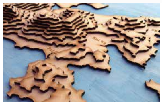
A laser cut model made from the 3D modelled data
