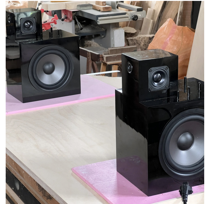
Cabinets with drivers installed
