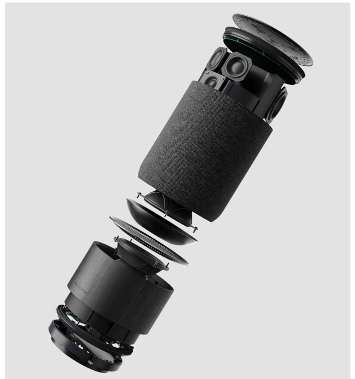
Internal structure image of Bang & Olufsen Beosound Balance (Force Cancelling)
